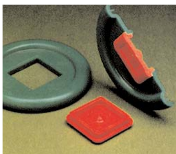
Sample disc and contrasting color insert provide good view of tight joint achieved via ultrasonic welding.
